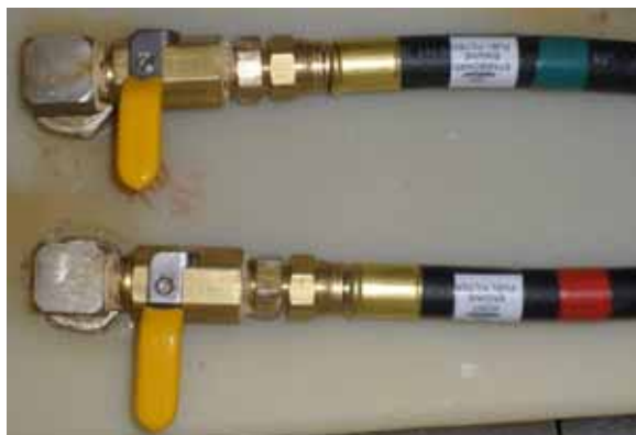
Fuel Tank Shut Off Valves
